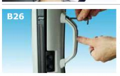
B26: (Assembly of the entry handles) It is now time to assemble both of the entry handles. Before screwing the handles, check if the wiring harnesses are not lying in front of the thread. If this is the case, press them carefully in the direction of the door seal with the aid of a suitable tool.
