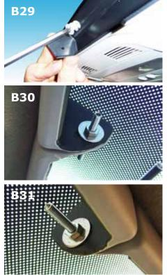
B29 - B31: (Assembly of the upper fascia panels) Attach the fascia panels with the accompanying wall plugs onto the roof lining. The set screw is screwed into the middle of the fascia panels on both sides with the accompanying pane and screws.
