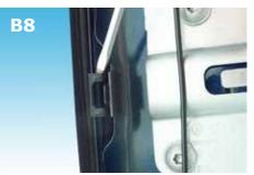
B8: (Disassembly of the fastening clips) Remove the metal clips from the vehicle panel by gently prying them from the anchorage with a flat object (e.g. a screwdriver).
