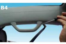
B4+B5: (Disassembly of the entry handles on the A-pillars) Loosen the entry handles' screws (TX 27) and remove them.
