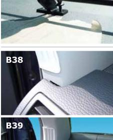
B38 - B40: (Attaching the foam strip) Under certain circumstances, different vehicle variants may lead to the formation of a gap between the dashboard and the A-pillar panelling (see B41). Cut the foam strip to match the size of the gap and stick it onto the A-pillar panelling.
