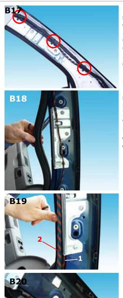
B17 - B20: (Positioning of the wiring harness (with rain sensor variant 2 wiring harnesses))
