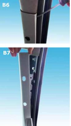
B6+B7: (Disassembly of the A-pillar panelling) Remove the original panelling above, beginning with the A-pillar. The clip-on connection automatically disengages in the process. Remove the panelling in an upward direction.
